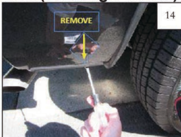
2012 Models Only (Optional): Remove inner piece at bottom rear of wheel well using a pry tool.
