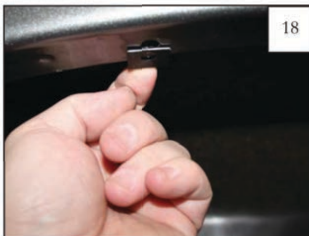
Install Clip (CL1-0022) over existing hole.
