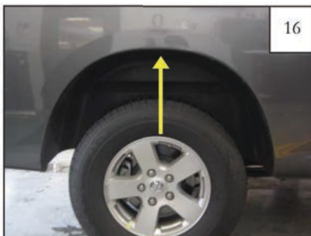
Install Clip (CL1-0022) in this location. See step 18.
