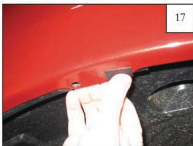
Install plastic tab over existing factory hole.
