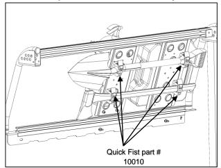
Using two Universal mounting plates and original Quick Fist you can mount a shovel and axe on inside
