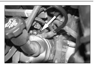
5. Disconnect crankcase vent hose from the valve cover as shown.
