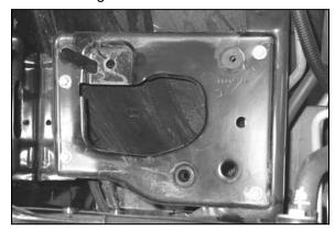
11b. Remove the heat shield assembly and drill a 5/8" hole through the marked location from step #11a.
