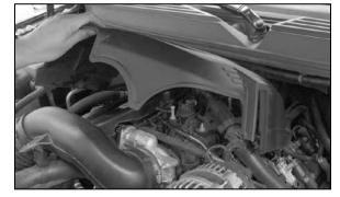
3. Lift up on the front of the engine cover to diengage from the mounting grommets. Then pull forward and remove the engine cover from the engine as shown.
