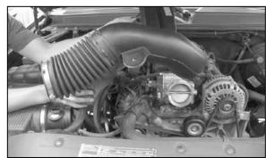
6. Loosen the hose clamps, which secure stock intake tube to the throttle body and mass air sensor and then remove the intake tube from the vehicle.
