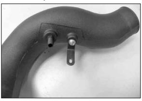
19. Install the "L" bracket (070812) onto the K&N® intake tube with the provided harware as shown.
