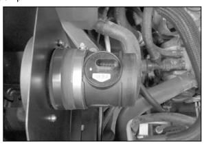
17. Install the mass air sensor assembly into the silicone hose on the filter adapter and secure with provided hose clamp.
