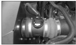
28. Reconnect the mass air sensor electrical connection.
