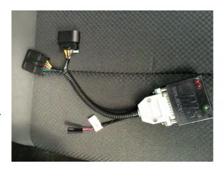
**Connect the Assembly:** Attach the black PedalMAX device to the wiring harness.
