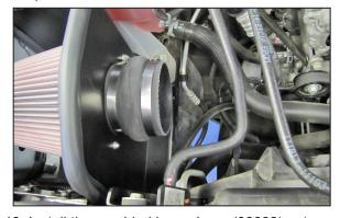
13. Install the provided hump hose (08699) onto the filter adapter and secure with the provided hose clamp.
