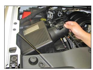
6. Lift up and remove the air filter housing from the vehicle.
