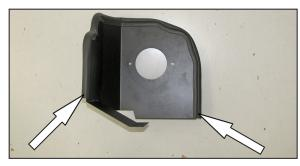
8. Install the provided edge trim onto the heat shield as shown.
