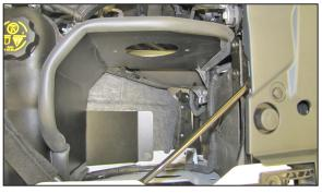
9. Install the heat shield and secure it to the air filter housing mounting plate location using three of the factory bolts from step #6.
