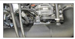
20. Reconnect the mass air sensor electrical connection.
