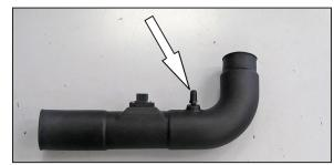
17. Install the vent fitting into the K&N® intake tube. NOTE: Plastic NPT fittings are easy to cross thread. Install the vent fitting "hand" tight, then turn it two complete turns with a wrench.
