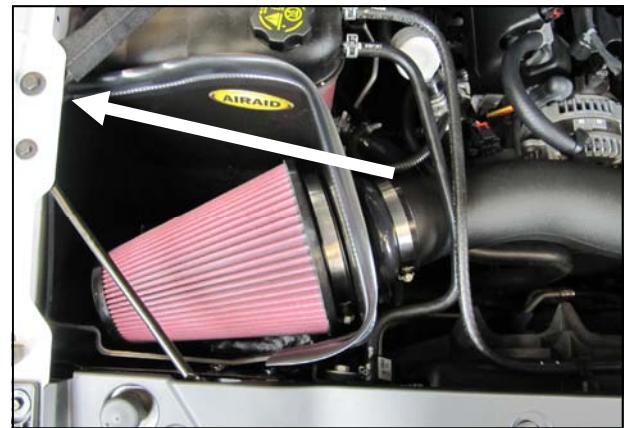
15. Reinstall the fender brace and the rear brace bolt. Make sure all clamps, hoses, bolts, and screws are tight. Double check the hood clearance. Reconnect the negative battery cable. The CARB Decal included with this kit must be placed in a conspicuous location under the hood in order to pass a Smog check.
