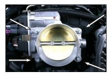
3. With a 10mm socket remove the two nuts, and the two bolts that hold the throttle body to the intake manifold. Without disconnecting the wiring harness, set the throttle body aside.
