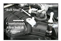
6. Remove the "ball stud" from the top of the intake manifold, insert the countersunk Allen bolt (#6) thru the countersunk hole in the provided 1" spacer plate (#5). Thread the countersunk bolt into the hole where you removed the "ball stud", face the spacer towards the front of the vehicle, and tighten the countersunk Allen bolt. Next thread the "ball stud" into the forward hole in the 1" spacer and tighten.
