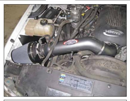
AEM® intake system installed
