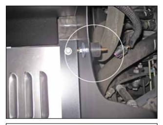
f. Install the rubber mount using the supplied washer and M6 nut on the heat shield.
