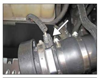
o. Reconnect the MAF sensor harness to the MAF sensor.
