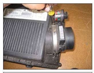
o. Loosen the hose clamp securing the MAF sensor to the stock air box. Remove the MAF sensor from the stock air box.
