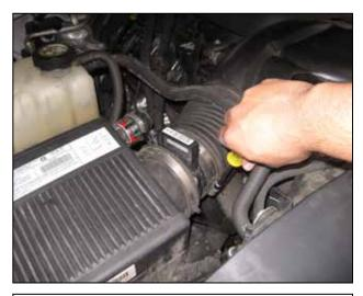
d. Loosen the hose clamp securing the intake duct to the MAF sensor.
