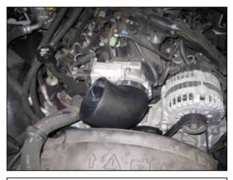
g. Install the 90° coupler on the throttle body and loosely secure with the supplied #64 hose clamp.
