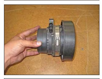
I. Assemble the MAF sensor and the supplied adapter as shown.
