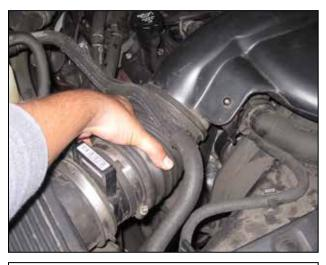
i. Disconnect the intake duct from the MAF sensor.
