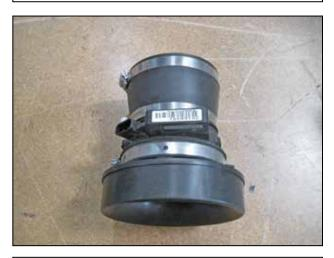
m. Attach the reducer coupler to the MAF sensor and secure with a supplied #64 hose clamp. Loosely attach another #64 hose clamp to the opposite end of the coupler.
