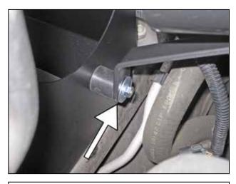
k. Install the supplied washer and the M6 nut.
