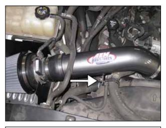
q. Secure the plastic mount on the radiator hose to the intake pipe.
