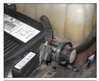
b. Disconnect the mass airflow (MAF) sensor harness.
