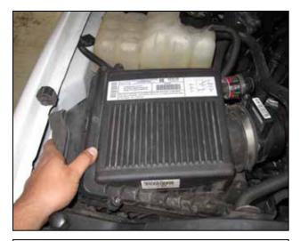
k. Pull up on the stock air box to disengage it from the plate on the bottom.
