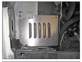
b. Place the splash shield in the location where the air box tray was and align the holes.
