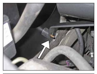
j. Align the bracket with the rubber mount installed in step 3(f).
