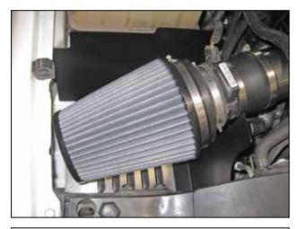
p. Install the air filter onto the adapter.
