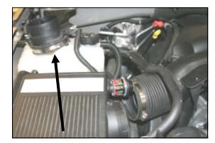
**3.** Without disconnecting the wiring harness, remove the Mass Air Sensor and coupler from the factory airbox, and set it aside.
