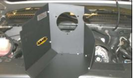
**4.** Grab the factory airbox and rock it back and forth, and remove it from the vehicle. It is only held in by grommets, no bolts.
