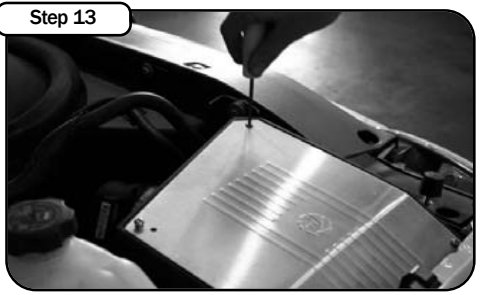
Step 13 Install housing cover onto box using supplied button head screws.
