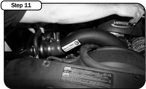
Step 11 Place straight coupler (05-00421) on throttle body and elbow coupler (05-00763) on tube. Slide tube onto throttle body coupler. Attach elbow to MAS. Tighten clamps. Rotate fan to ensure sufficient clearance.
