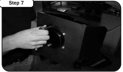
Step 7 Place the air filter adaptor inside the housing. Secure the adaptor with the supplied screws and washers.
