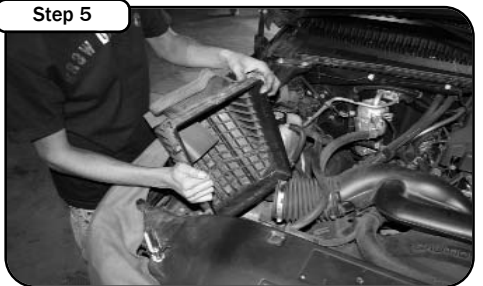
Step 5 Grab the lower portion of the airbox then lift up and out. The box is secured with rubber gromets.
