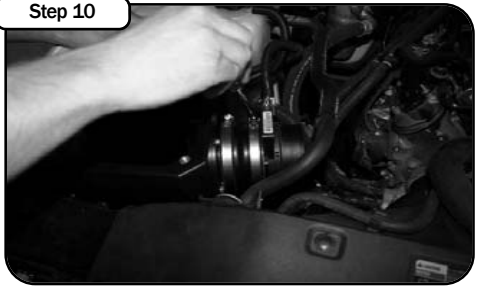
Step 10 Install MAS using supplied clamps and reducer coupler (05-00020). Do not tighten clamps at this time.
