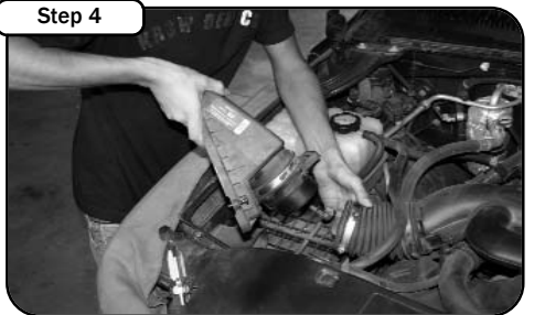
Step 4 Loosen the hose clamp connecting the MAF sensor to the airbox. Remove upper portion of the airbox and MAF sensor. Carefully set to the side for later use.
