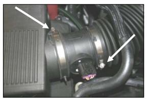
1. <u>Disconnect the negative battery cable.</u> Loosen the hose clamp on the end of the factory intake tube at the Mass Air Flow sensor, next loosen the hose clamp that holds the Mass Air Flow sensor to the factory air box.
