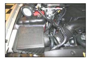
**3.** Without disconnecting the wiring harness, set the Mass Air Flow sensor out of the work area. Next rock the factory air box back and forth, lift it up, and remove it from the hold down grommets. There are no bolts holding it down.
