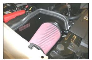
**10.** Install the Airaid Premium Filter (#1) onto the filter adapter (#4), and tighten the hose clamp. Next install the weather strip (#5) onto the top of the **CAD** as shown. For ease of installation start at the fender, and work towards the radiator.
