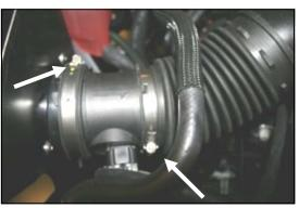
**9.** Re-install the Mass Air Flow sensor and coupler onto the air filter adapter (#4), as shown and tighten the hose clamp. Next re-connect the factory intake tube to the Mass Air Flow sensor, and tighten the hose clamp.
