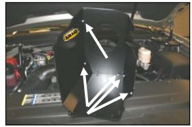
**6.** Assemble the two Cool Air Dam panels (#2) and (#3) using the five supplied screws (#9), washers (#10), and nuts (#11). Apply the Airaid Foil Decal onto the Panel as shown.
