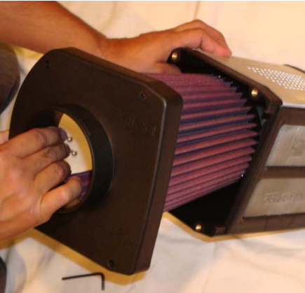
Pull the velocity stack base with the filter that is attached to the velocity stack.
