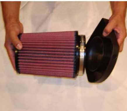
Once you have loosened the filter neck clamp, continue to pull the filter from the velocity stack,
