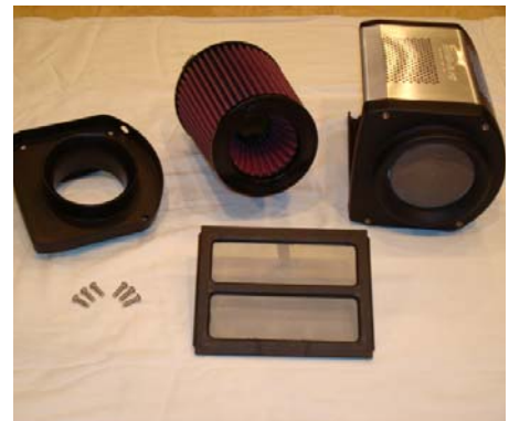
Here is a group shot of the components that goes into the power-box. The filter and screens can now be cleaned with a simple shop-vac.
