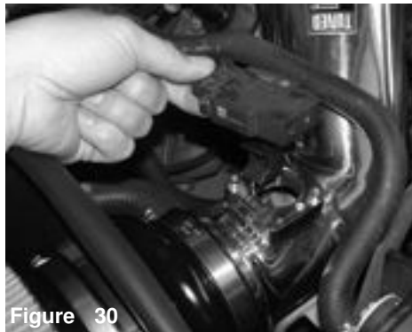
Figure 27 Now firmly push the sleeve hose end of the intake pipe onto the throttlebody
