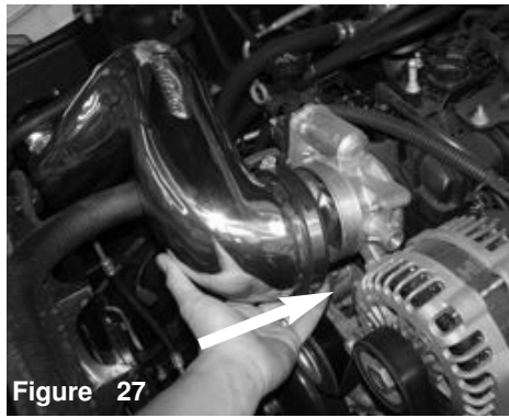
Figure 26 Place the MAF sensor end into the 4.0" hump hose.
