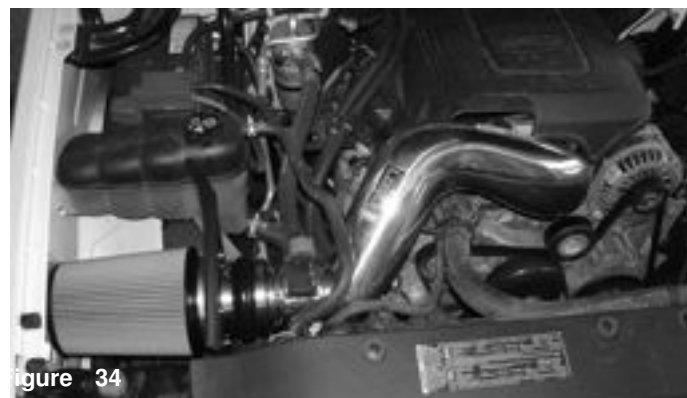
Figure 32 Re-connect the MAF sensor harness to the MAF sensor.
