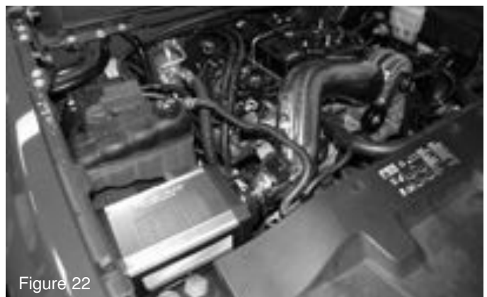
Press the Injen 9"-10mm vacuum crank case line over the cast tube vacuum port and the port on the valve cover
