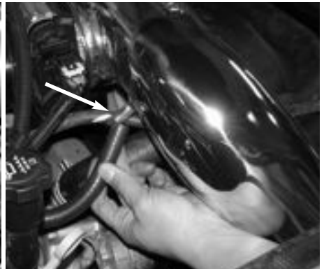
Press the Injen 9"-10mm vacuum crank case line over the cast tube vacuum port and the port on the valve cover
