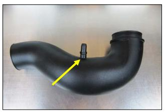
3. Install the Barbed Fitting into the Intake Tube as shown.
