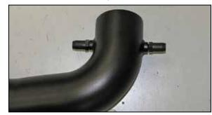
17. Install the two provided crank case vent fittings into the K&N<sup>®</sup> intake tube as shown. NOTE: Plastic NPT fittings are easy to cross
