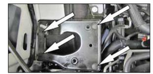
7. Remove the four bolts securing the air box mounting tray and then remove the tray from the vehicle.
