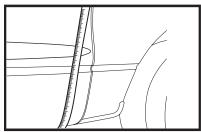
3. After confirming you have the correct length moldings, mask off a straight section on the door to use as a guide to aid in installing the moldings straight and level. Take into consideration clearance needed to open door. (2 inches)
