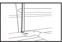
4. Confirming masking tape is straight and level. With tape measure, measure vertically along door. Lengths should be the same along both sides of tape. Use horizontal centerline of each molding piece. If heights are different make adjustments until they are equal in length.
