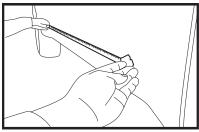
2. Determine location of where universal Body Side Moldings will be placed. Moldings must only be installed on a flat non curved section of the door to adhere properly. Only measure the flat non curved section of the door and determine if you have the correct length moldings before proceeding. Allow no more than 2 inches of clearance on each end of the Body Side Moldings to door edge for optimal clearance and appearance.
