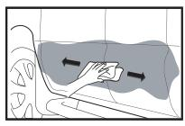
1. Wipe down surface with a soft towel soaked with alcohol to remove any wax or contaminants from paint finish of vehicle's lower door area.
