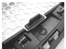
12. Use pliers to snap in black plastic clips from the kit to every tab location on top and bottom grille insert. Thinner side of clip goes toward grille opening.
