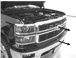
Pull grille and upper bumper pieces out away from truck and place face down on scratch free surface. These two pieces will be attached together.
