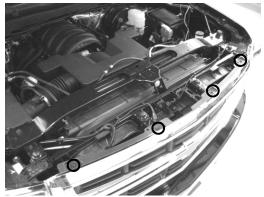
Once cover is removed, remove the top 4 grille screws with 10mm wrench (location shown above).
