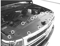
Remove plastic cover by removing 12 retaining clips with flat head screw driver (locations shown above).
