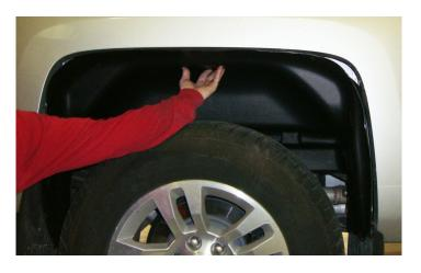
5. Push The Wheel Well Guard up into the wheel well opening.
