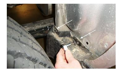
2. Reinstall 2 factory screws that hold the factory rock guard on the front side of the fender and tighten.(2 places per side)
