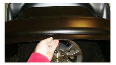
4. Insert the Wheel Well Guard into the rear wheel well opening over the tire.
