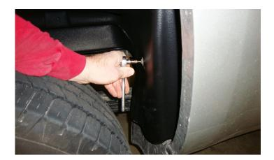
8. Align the 4 holes in the Wheel Well Guard with the factory screw locations and install the factory torx head screws. Install all screws before tighting.
