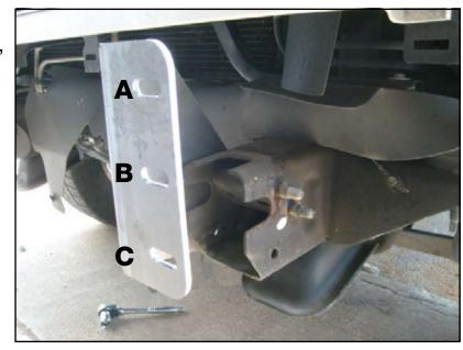
ALIGN THE BUMPER SIDE TO SIDE AND TOP TO BOTTOM TO ENSURE A PERFECT FIT TO THE TRUCK. ALLOWFOR A 0.25" CLEARANCE TO ALL PAINTED SURFACES IF POSSIBLE TO ALLOW FOR FRAME FLEX.
