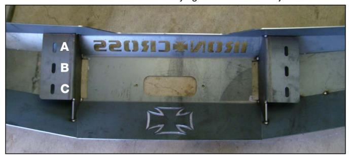
Install 1/2" hex bolt, (2x) 1/2" flat washers, 1/2" lock washer, and 1/2" hex nut into holes A, B, & C through bumper and bumper brackets.
