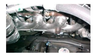
8) REMOVE THE SIX BOLTS ATTACHING THE MANIFOLD TO THE HEAD. REMOVE THE MANIFOLD.CLEAN THE SURFACE OF THE HEAD. REMOVE ANY CARBON DEPOSITS THAT MAY BE ON THE HEAD.PREPARE THE SUPPLIED HEADER BOLTS WITH ANTI-SEIZE TO THE THREADS.
