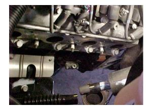
3) **MARK ALIGNMENT OF THE SHAFT BEFORE REMOVING,** THEN REMOVE THE BOLT FROM THE STEERING SHAFT. SLIP STEERING SHAFT APART. NOW UNBOLT THE MANIFOLDS FROM THE STOCK EXHAUST SYSTEM.
