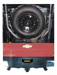
8. Install exit pipes #E onto tailpipes. Cut to your preferred length then use clamps to secure exit pipes to tailpipes. Install stainless steel tips. Clamp down. When you have everything in place, firmly tighten all bolts and clamps down securely. Use stainless steel cleaner and a Scotch Brite pad weekly to prevent tip from discoloration. Inspect all fasteners after 25-50 miles of operation and re-tighten as necessary.
