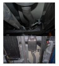
4. Install muffler #B with inlet towards Y-pipe. Use jack stands to support the muffler. Use clamp #F to secure the muffler to headpipe. Do not tighten.
