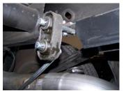
5. Next, remove your spare tire. Then install passenger side tailpipe hanger #I. You will see a 11/2" hole in the frame. Attach hanger to this hole and re-install factory grommet on hanger.
