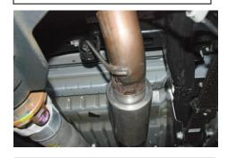
5. With everything loose you may need to adjust the system for proper clearance of shocks, brake lines, ect.
