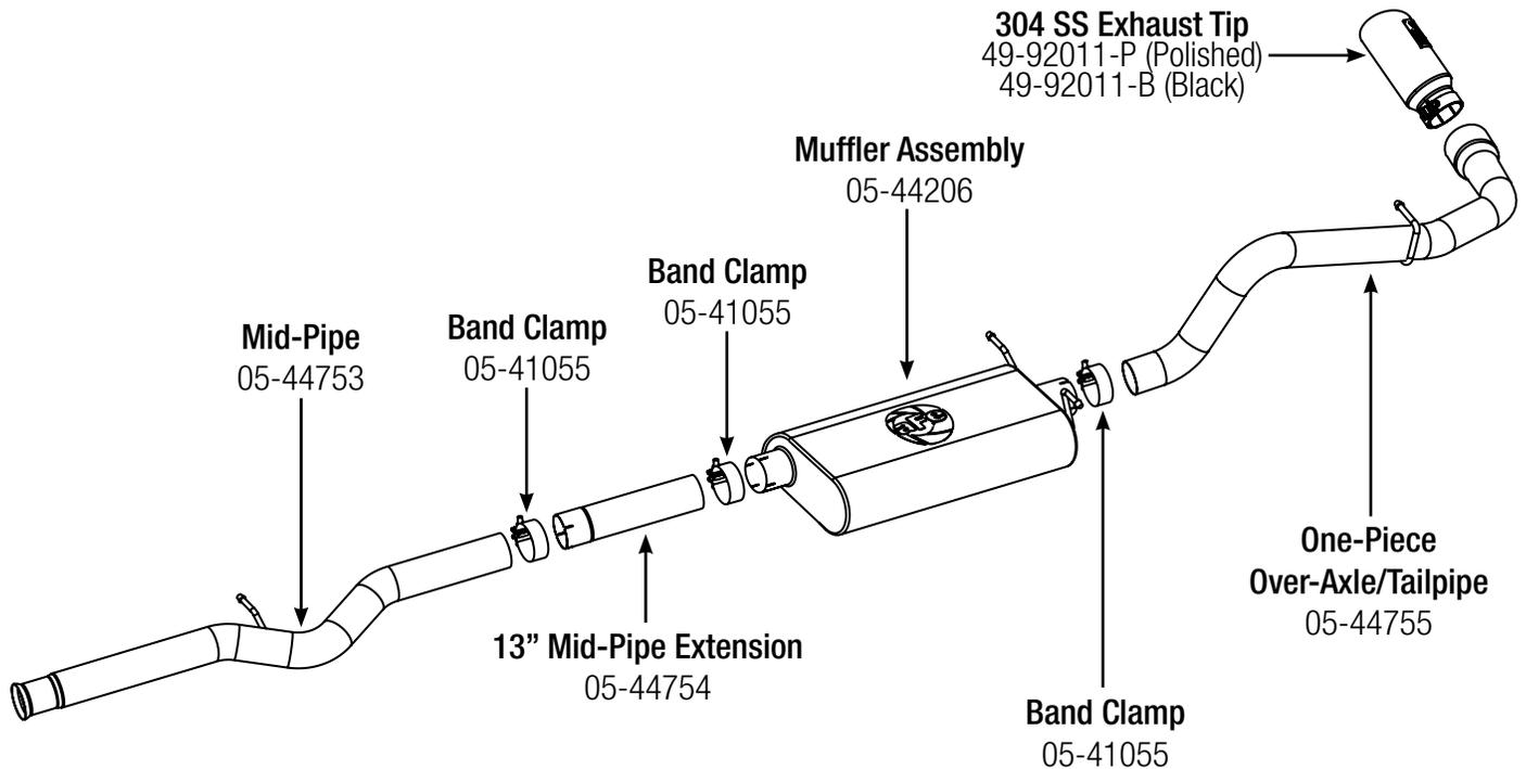
**Step 1: (Read Instructions prior to installation)** Remove your stock exhaust up to the catalytic converter from the rear of your truck working your way forward. Take caution not to damage the factory hardware and isolation mounts as they will be reused.
