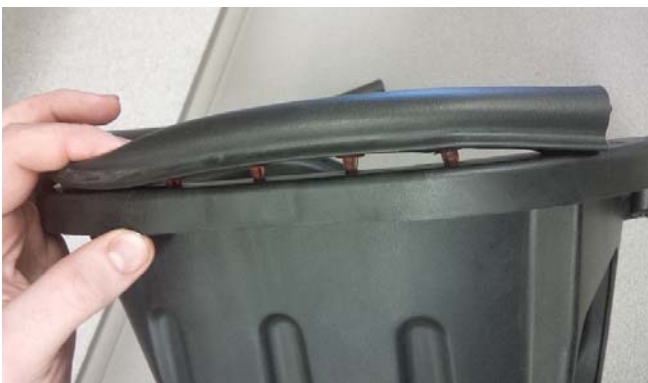
6. Clean off the fender well, then attach the inlet seal (P/N: 2414-9F673) as shown.
