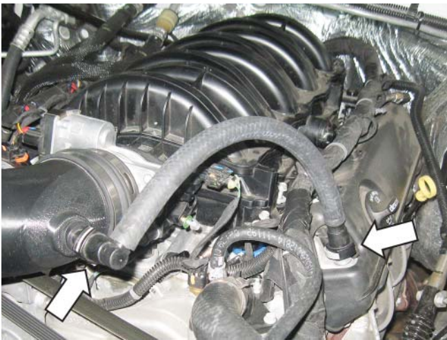
16. Install the passenger side PCV hose (P/N: 2414-6757) between the quick connect bars on the valve cover and clean air tube assembly.
