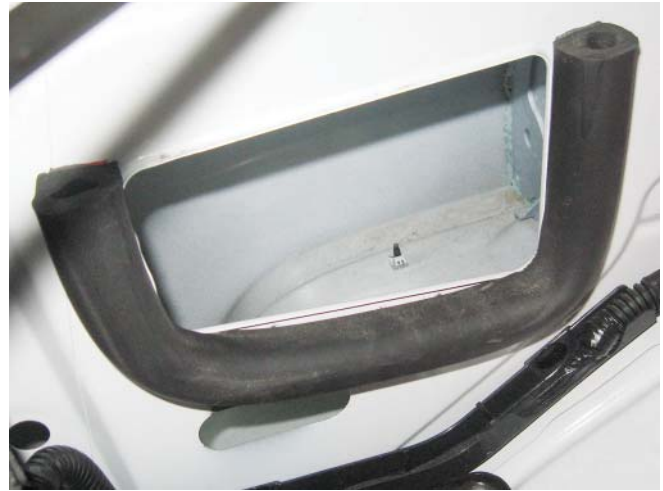
7. Insert the air box assembly into the truck, push down to seat the posts into the grommets.
