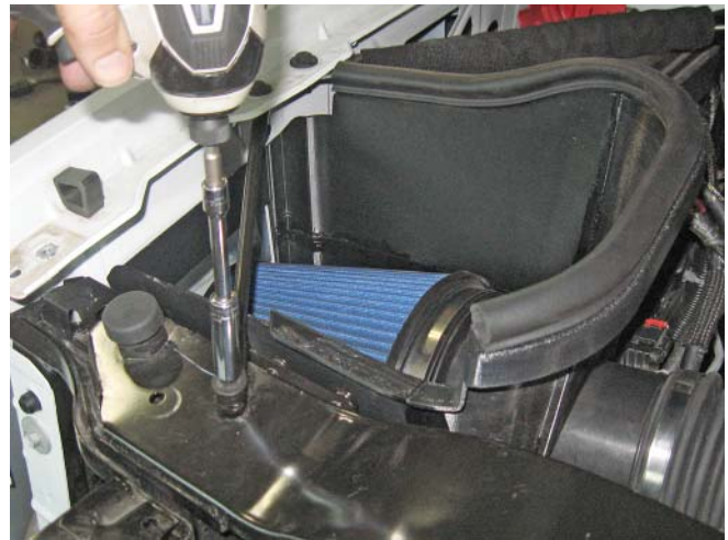
17. Reinstall the support brace between the core support and fender.
