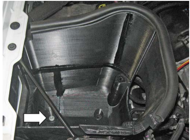
8. Thread and tighten the provided M6 bolt (P/N: N605891) into the bottom of the air box. Tighten to 10 Nm.
