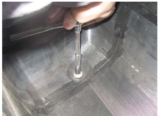
8. Thread and tighten the provided M6 bolt (P/N: N605891) into the bottom of the air box. Tighten to 10 Nm.
