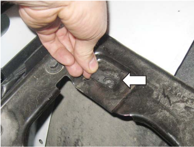
4. Install the grommet (P/N: 9600K53) into the air box tray as shown.
