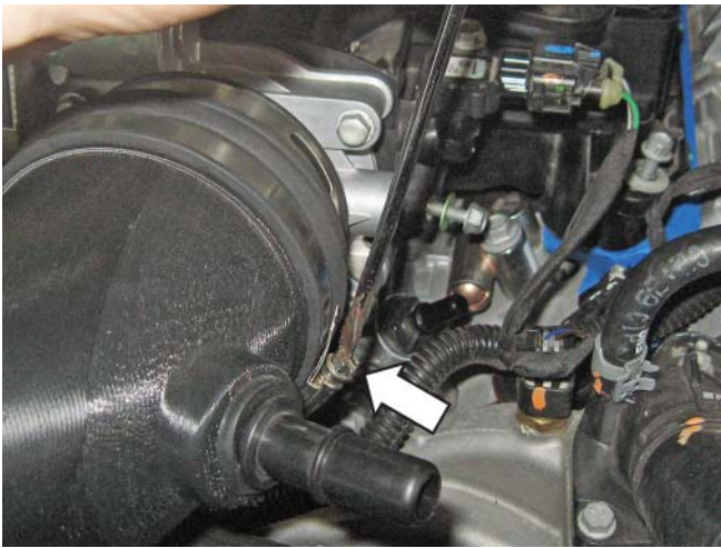
15. Install the driver side PCV hose (P/N: 2414-6758) between the quick connect bars on the valve cover and clean air tube assembly.
