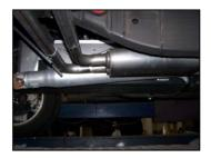
4. Slide the muffler assembly into the headpipe at least 1.5"-2". Use a jack stand to support the muffler assembly. Use clamp #E to secure muffler assembly to the headpipe. Do not tighten. Insert welded hangers into rubber grommets.
