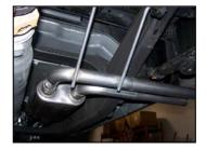
5. Rotate the muffler assembly until the outlets are level.
