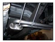
5. Rotate the muffler assembly until the outlets are level.
