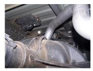
6. Install driver side tailpipe #D into muffler at least 1.5" to 2". This pipe will route over the axle and between the shock and spare tire. Use clamp #G to secure pipe to muffler. Do not tighten. Insert welded hangers into rubber grommet.
