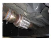
unclamp it at the ball flange behind the Y-pipe. Make sure to leave all rubber grommets in the factory location. **You will re-use stock clamp.** For easier removal of exhaust, cut behind the muffler. Use WD-40 to remove hangers from grommets.
