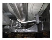
Bolt head pipe #A to the Factory pipe. Insert welded hanger into rubber grommet. Do not tighten.
