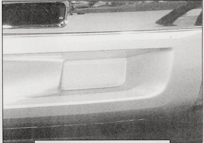
(Fig 2) No opening in bumper cover
