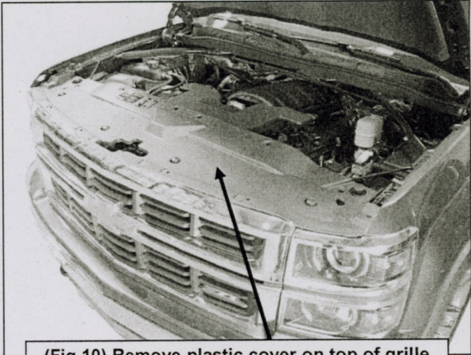
(Fig 10) Remove plastic cover on top of grille
