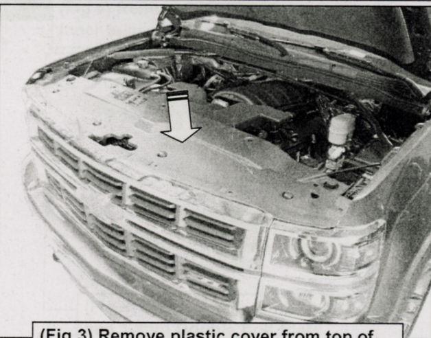
(Fig 3) Remove plastic cover from top of radiator (arrow). Temporarily remove grille
