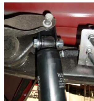
60. Install shock with extension into upper mount (leave Loose).
