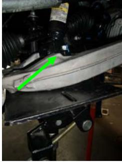
32. Raise lower control arm to attach strut & torque.
