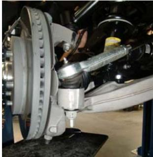
36. Re-attach the tie rod and torque.
