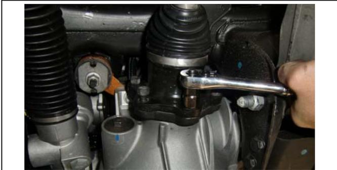
39. Reconnect Inner CV flange torque.
