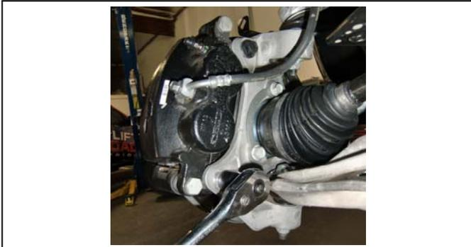
37. Re-attach caliper & torque. **Repeat 29-37 on other side.**
