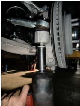
9. Loosen tie rod and remove from knuckle.
