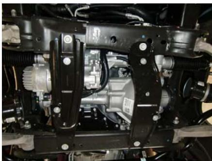
19. Remove plastic air dam tin mounting brackets.
