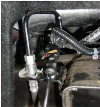
41. Reconnect ABS lines and attach in factory location.
