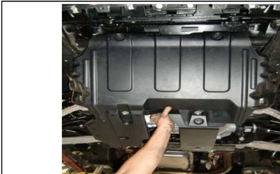
47. Test fit to ensure fit and finish.
