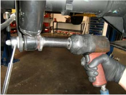
61. Install shock into lower mount and tighten.
