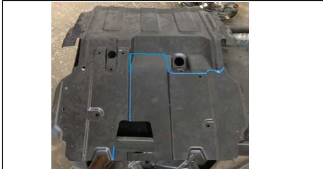
45. Cut lines marked on air dam.
