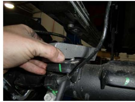
54. Lower axle and remove factory blocks.
