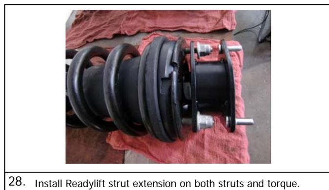
28. Install Readylift strut extension on both struts and torque.
