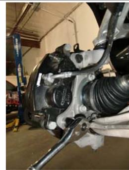
8. Remove caliper & secure to vehicle out of the way.
