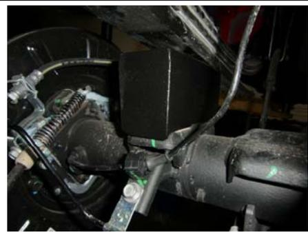
56. Raise axle to engage lift blocks and centering pins.
