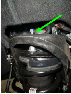
31. Install strut with spacer leaving nuts loose.
