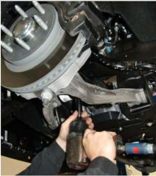
13. Loosen and remove bolts from lower strut mount.
