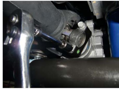
38. Re-attach front drive shaft using OEM bolts and straps.
