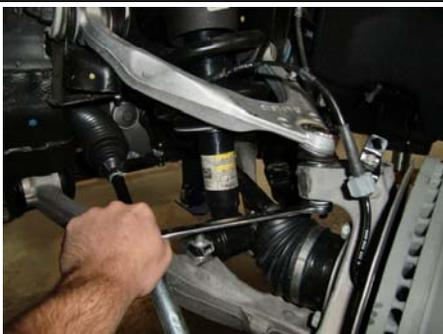
11. Loosen & separate ball joint from knuckle.
