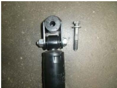
59. Install shock extensions to the top of the shocks (for OEM shocks only).
