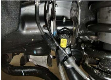
40. Reconnect brake line to control arm using new hardware.
