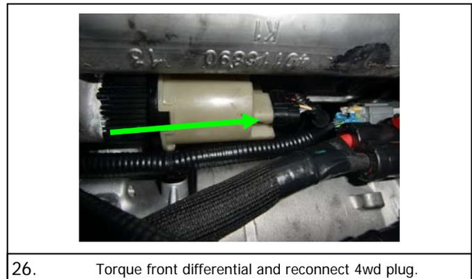
26. Torque front differential and reconnect 4wd plug.
