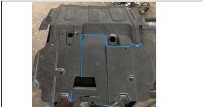
45. Cut lines marked on air dam.
