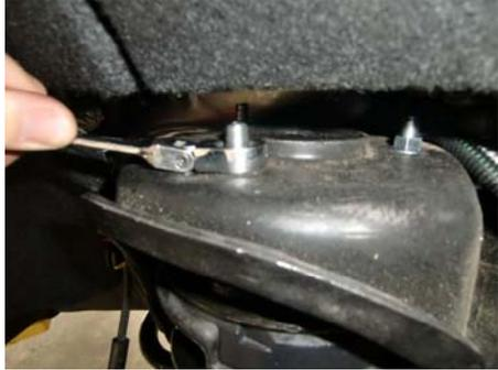
34. Once the lower is tightened, torque the top nuts.
