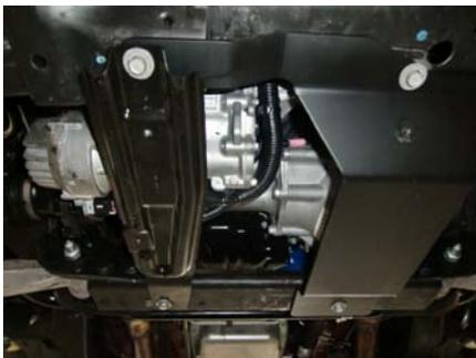
43. Re-attach passenger side sheet metal for air dam mount.
