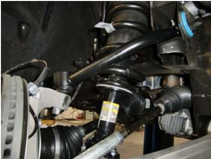
35. Connect upper control arm to knuckle and torque.
