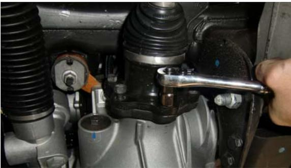
39. Reconnect Inner CV flange torque.
