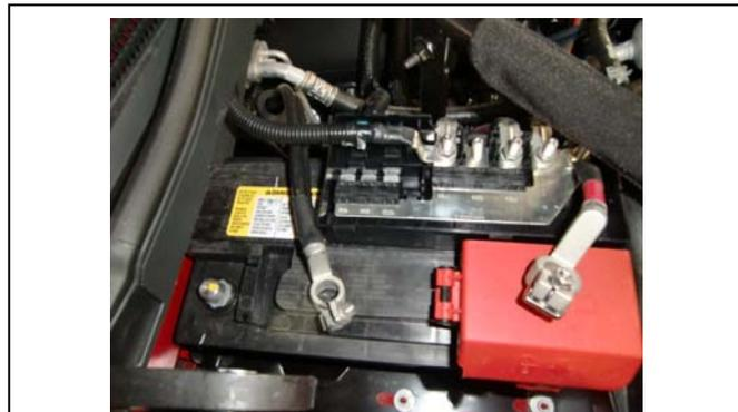
3. Disconnect battery connections.
