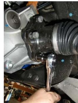
10. Remove bolts from inner CV drive flange.
