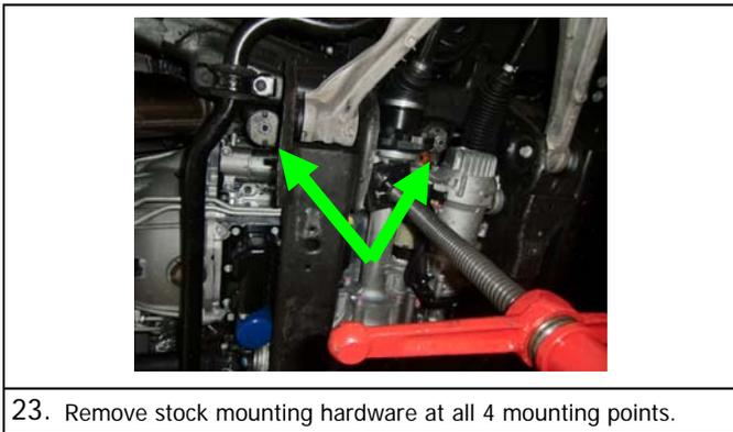
23. Remove stock mounting hardware at all 4 mounting points.
