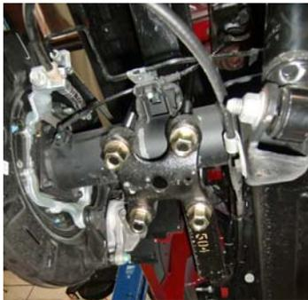
57. Install new hardware and factory axle plate.
