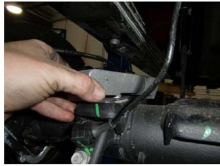
54. Lower axle and remove factory blocks.
