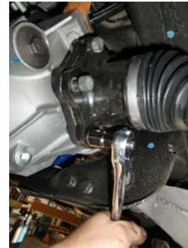
10. Remove bolts from inner CV drive flange.
