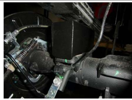
56. Raise axle to engage lift blocks and centering pins.
