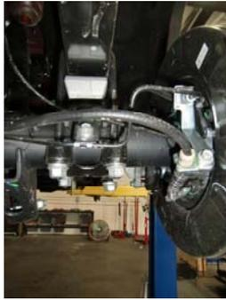
53. Remove U-Bolts, axle plate (one side at a time).
