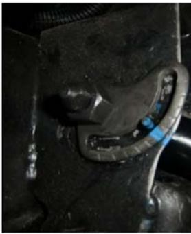
15. Mark alignment cams & note direction/location of hardware.
