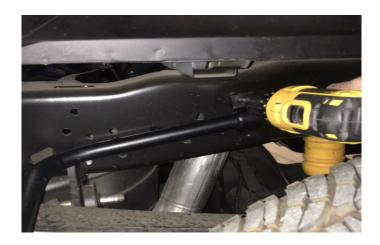
4. Use supplied self drilling screws and washers to fasten the mounting bar to the frame.
