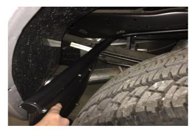
5. Slide the mud flap and flange over the mounting bar and tighten the bolt to hold the mudguard at your desired angle
