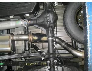
**Step 3.** Install the Muffler to the Inlet Pipe Assembly using the supplied 3.50" clamp. Next install the over axle Resonator assembly to the Muffler in the similar fashion using the supplied 3.50" clamp, fitting the welded hangers into the rubber insulators.
