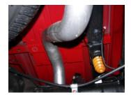
5. Install the overaxle tailpipe #C onto the outlet of the muffler 1.5"-2" using clamp #E to secure pipe to muffler. Insert welded hanger into rubber grommet.
