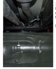
3. Bolt adapter #I to the stock flange re-using the factory into rubber grommet. Do not tighten.
