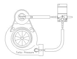
Hookup for Internal Wastegates: Port 1: Sintered Muffler
