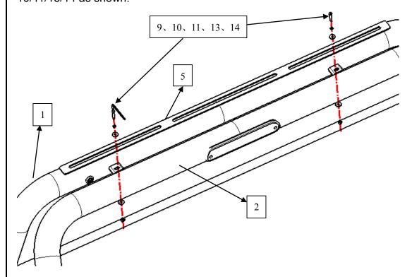
Step3: Using wrench 9, install 3/4 decoration plate together with parts 10/11/13/15 as shown.
