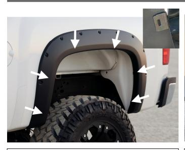
**STEP 11:** To secure the Fender Flare to the body, take the black metal clips and slide them over the Fender Flare and the inner wheel arch lip. Position the clip so that the barb in the clip locates in the slot of the Fender Flare. Ensure all fixing points are secure and that the rubber seal is flush neatly against the body.
