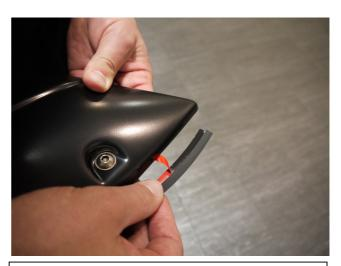
**STEP 8:** Attach the included rubber seal to the Fender Flares. Peel back 2" of the adhesive backing and position on the Fender Flare. Attach the seal to the Fender Flare, peeling back a few inches at a time. Ensure pressure is used to secure rubber seal to Fender Flare edge. Attach rubber seal along all areas the Fender Flare will make contact with the vehicle body.
