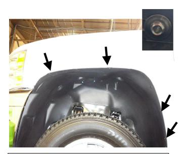
**STEP 5:** Place the Fender Flare on the vehicle into the position of best fit. Note where the slots in Fender Flare at positions **A**, **B**, **C**, **and D** align with the existing screws in the vehicle. Remove Fender Flare. Use the original manufacturer's hardware that is in the wheel arch of the vehicle to fit the Fender flares. Remove the x4 9/32" (7mm) socket head screws from the fasteners on the vehicle.
