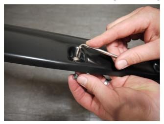
**STEP 7:** Attach the 11 bolts, washers and nuts to each Fender Flare using a 5/32" Allen key and a 3/8" wrench/socket. (wrench/socket and Allen key not supplied). Ensure inside of Fender Flares where the rubber seal is attached is clean, using the alcohol wipes provided. Wipe away any residue with a dry clean cloth.
