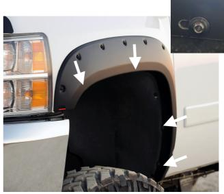
**STEP 6:** Place the front Fender Flares onto the vehicle and line up the holes on the part with screw holes on the vehicle. Re-Install the socket head screws into the fender to secure the Fender Flares. Fit the Fender Flares loosely until the Fender Flares are aligned as desired, when satisfied tighten the screws fully to ensure rubber seal is flush neatly against the body.
