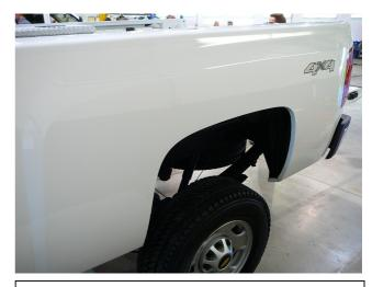
**STEP 10:** Clean the body areas where the Fender Flares will make contact. Ensure fenders are dry prior to install.
