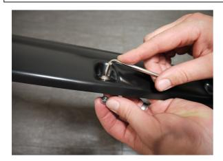
**STEP 1:** Attach the 9 bolts, washers and nuts to each Fender Flare using a 5/32" Allen key and a 3/8" wrench/socket. (wrench/socket and Allen key not supplied). Ensure inside of Fender Flares where the rubber seal is attached is clean, using the alcohol wipes provided. Wipe away any residue with a dry clean cloth.
