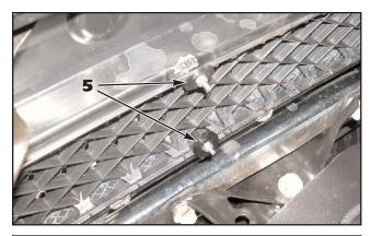
Carefully install large black plastic washers and #8-32 ESNA nuts onto the studs and but do not tighten until the protective masking tape is removed from the factory grille frame.
