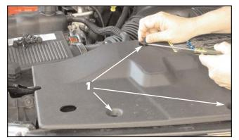
1. Open the hood and remove all the factory push pins securing the cover from the top of the radiator support panel.
