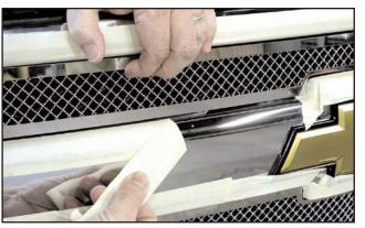
**6**. Carefully peel off the protective masking tape from the factory grille frame (pull it back over itself as shown to minimize breakage, you can also shift the mesh grille sections to create additional clearance).
