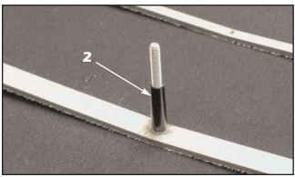
2. Cut the end from each black silicone sleeve and install one onto the bottom and side studs on the upper and lower grilles prior to vehicle installation (lower shown).
