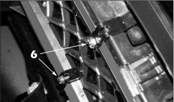
6. Carefully align the supplied U-shaped mesh retainers to all mounting studs and install the supplied #8-32 ESNA half nuts onto the studs and tighten until the grille is snug. Do not over tighten or you will indent the grille at the stud locations.
