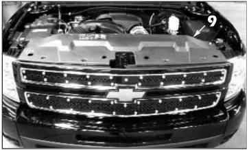
**9.** Reinstall the radiator support panel cover once all mounting hardware has been tightened and close the hood. Clean grille to remove fingerprints, grease, etc.
