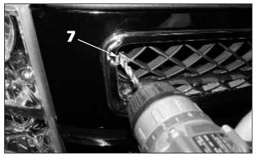
**7**. Prior to upper upper mesh grille alignment, use a 5/16" drill bit to enlarge the existing opening in the factory grille where shown.
