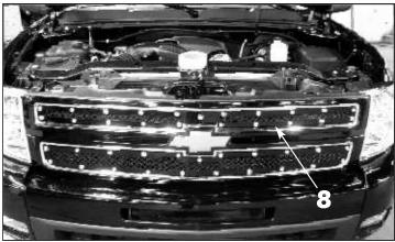
**8.** Install the upper upper grille using the same procedure as the lower upper grille.
