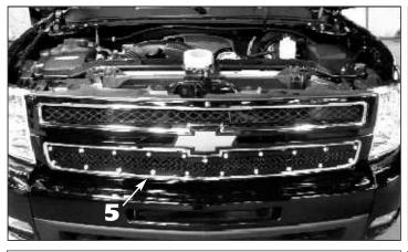
**5**. Align the lower upper grille assembly into place, making sure the studs pass through the openings in the factory grille.
