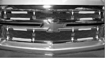
**4.** This photo shows the screw and 4-way mesh retainer locatons that will secure the mesh sections to the factory grille inserts.
