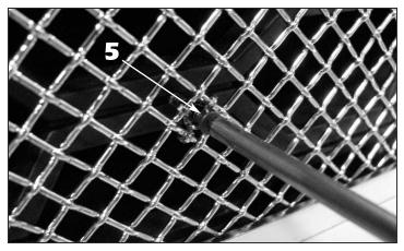
5. Carefully align the supplied 4-way mesh retainers and install the supplied #4 x 3/4" screws painted in step 1 through the centers of the thickest parts of the factory grille insert. You can use a 1/16" drill bit to drill the mounting holes or allow the screws to self-tap into the factory grille inserts.
