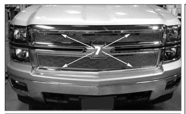
7. Remove the masking tape and clean grille to remove fingerprints, grease, etc. Use a mild solvent and a soft, clean cloth to remove any glue residue from the polished stainless steel surrounds. Follow with alcohol or glass cleaner and a soft, clean cloth to remove any solvent residue. Finished installation.
