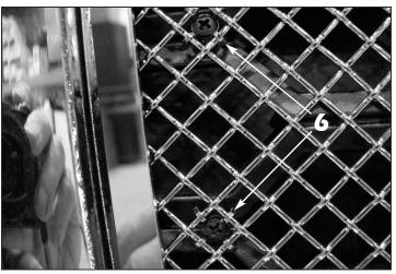
**6**. Image shows proper placement of the 4-way mesh retainers and mounting screws installed through the thickest part of the factory grille inserts. Do not overtighten or you will strip out the holes in the factory grille inserts!
