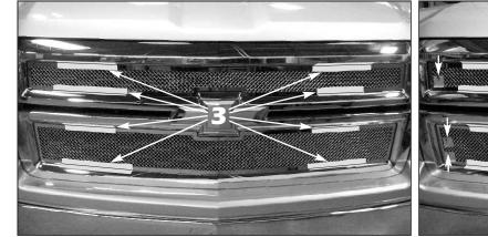
Align the grille assemblies into place and use enough wide masking tape to hold them in place for the following hardware installation.
