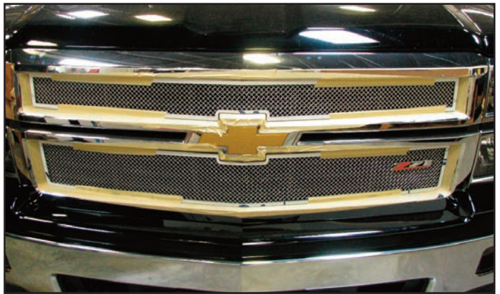
8. Align the mesh grilles into place and use wide masking tape to hold them in position for the following mounting hardware installation. Make sure the emblem mounting studs do not make contact with the factory grille (mesh grille shown, E-Power mesh grille similar).
