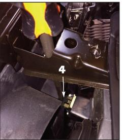
**4**. Use a long, flat blade screwdriver or pry bar to release the side and lower clips retaining the bottom of the factory grille.
