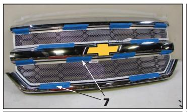
**7**. Align the grille assemblies over the factory grille, making sure the mounting studs pass through the holes drilled in the previous step. Once the grilles are prefectly centered, use wide masking tape to hold the grilles in place for the following hardware installation.
