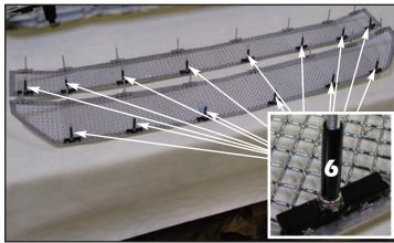
6. Trim the closed ends form the preinstalled black cap plugs and reinstall the caps onto the bottom mounting studs on the mesh grille sections (chrome mesh shown, "Black Ice" and "Stacked" grille procedure is the same).
