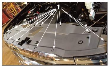
Remove the twelve factory push pins from the radiator support panel cover and remove the cover for factory grille mounting hardware access.
