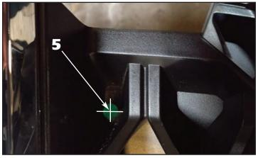
**5.** The outer mounting holes for the mesh grilles will need to be drilled through the air flow panel behind the grille using a 5/16" drill bit at the inner corner recesses of the factory grille (see arrow). A total of 6 holes need to be drilled.
