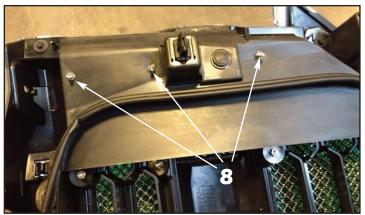
Install the #8-32 ESNA half nuts and tighten until the grille is tight against the factory insert. You will not need washers, the black out panel will work for these six studs..
