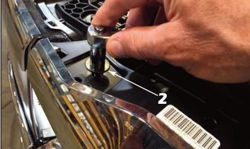
**2**. Remove the four upper 10mm bolts retaining the factory grille to the core support.
