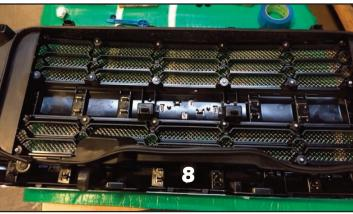
**8.** Place the grille faced down and install the supplied large black plastic washers and #8-32 ESNA half nuts and tighten until the washers no longer freely rotate.
