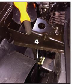
blade screwdriver or pry bar to release the lower clips retaining the bottom of the factory grille.
