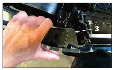
**3**. Lift up on the factory grille and pull the grille forward to release the top of the grille from the core support.
