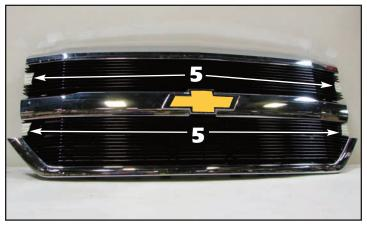
**5**. Align the grilles into place, making sure that they are prefectly centered. Use wide masking tape at the edges to hold the grilles in proper alignment (see arrows), then turn the grille assembly face down for mounting hardware installation.
