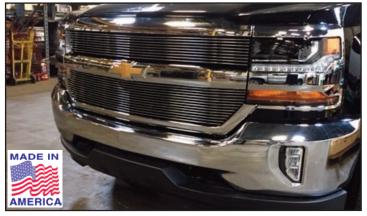
Reinstall the grille assembly by reversing Steps 1-4. Remove the masking tape and clean the grille to finish the installation.
