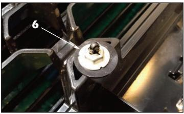
**6**. Install the large black plastic washers and 3/16" speed nuts over the protruding studs and tighten until the grille sections are tight against the factory grille.
