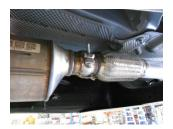
1) Place inlet pipe assembly #26429S into position onto the ball connection behind the catalytic converter. Reinstall the clamp onto the ball connection and tighten enough to hold, but still allow for a small amount of adjustment. Connect the hanger on the pipe to the rubber mount on the vehicle.
