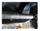
2) If installing the system on a Crew Cab truck with a 6.5' bed, place extension pipe **#TB700S** onto the back of the **#26401S** inlet pipe, place a provided clamp onto the slip-fit and tighten enough to hold in position. The extension pipe will not be used on Double Cab-6.5' bed or Crew Cab-5.5' bed models.
