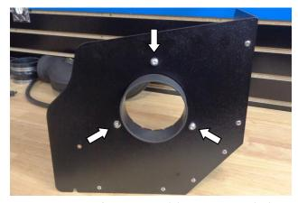
15. Assemble air filter adapter (3) to heat shield (18) using M6 screws (7), lock washers (6) and flat washers (5).
