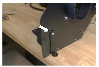
16. Attach long bracket (16) to heat shield using ¼-20 screw (15) (against the bracket) and nut (21), lock washer (20) and flat washer (19) (against the heat shield). Do not fully tighten hardware at this time.
