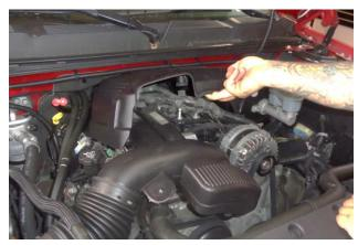
4. Remove the engine cover by firmly lifting it straight up to release it from its friction clips.
