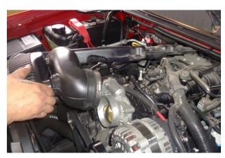
11. Disconnect the intake duct from the throttle body, and remove the duct from the vehicle.
