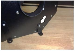
17. Attach short bracket (17) to heat shield using ¼-20 screw (15) (against the bracket) and nut (21), lock washer (20) and flat washer (19) (against the heat shield). Do not fully tighten hardware at this time.
