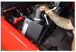
12. Remove the assembled airbox and MAF sensor by grasping the sensor and lifting straight up (to release the airbox mount pins from their rubber grommets), then sliding the airbox inboard to release it from its shelf.
