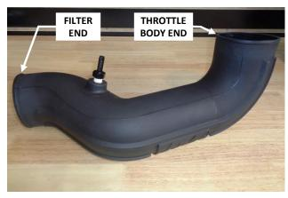
21. Apply 2 wraps of nylon thread tape to threads of 3/8" barbed fitting (9), and install it in the intake tube (13). Note the Filter and Throttle Body ends of the tube (for the next two steps).
