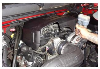
31. Install the engine cover by aligning it with its mount posts, then snapping it into place.
