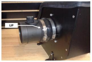
19. Slip two hose clamps (8) onto a 3¾" - 4" coupler (14). Push the coupler's 4" end onto the air filter adapter, all the way against the heat shield, and tighten the clamp. Orient the MAF sensor so that the airflow arrow points away from the coupler, and push the sensor fully into the coupler, so that its lip touches the coupler, then tighten the clamp.
