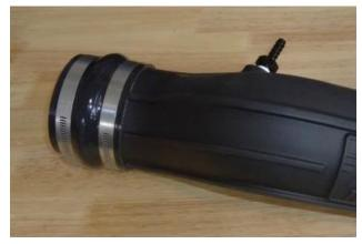
22. Slip two hose clamps (8) onto the other 3¾" - 4" coupler (14). Install the 4" end of the coupler on the Filter end of the intake tube, and snug (but do not yet tighten) the hose clamps.
