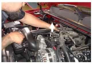
10. Lift the intake duct resonating chamber straight up, just enough to release it from its friction clip.
