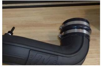
23. Slip the last two hose clamps (8) onto the 4" coupler (12), then install the coupler on the throttle-body end of the intake tube. Snug (but do not yet tighten) the clamps.
