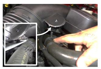
5. Use a flat-tip screwdriver to separate the coolant hose clamp from the intake duct, then remove the clamp from the hose.
