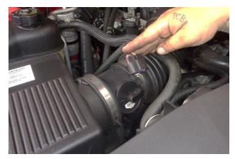
6. Disconnect the electrical plug from the Mass Airflow (MAF) sensor.
