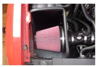
30. Slip clamp (2) onto air filter (1), install filter on filter adapter, and tighten clamp.
