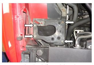
14. Remove the airbox shelf mount bolts, and remove the shelf. Retain the bolts for installation of the heat shield at Step 20. NOTE: During removal of airbox shelf mount bolts, if there are any differences in bolt length, note each bolt's location, in order to maintain proper hardware clearance at reinstallation.
