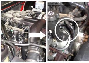
9. Carefully pull the breather hose off the breather line (just inboard of the oil filler neck – shown disconnected).
