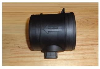
13. Remove the MAF sensor from the airbox.
